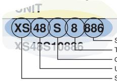
Spacing Frame Heights Table Frame Height Construction Material\* Unit Diameter Separator Model
