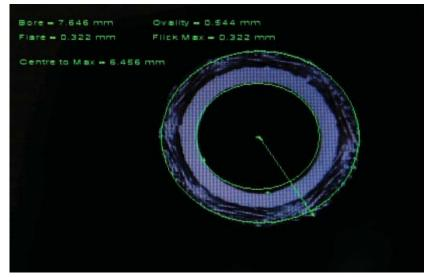
In addition, Aflex have developed a fully automated inspection system which checks the cut ends for diameters, ovality and protruding cut wire ends.
