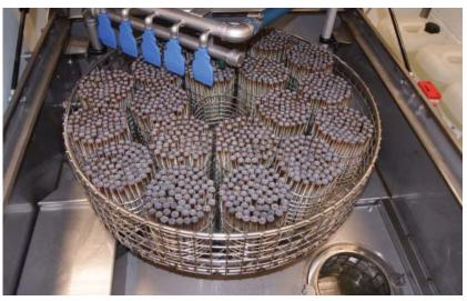
Automated washing equipment is available for short cut lengths, capable of achieving the required tolerance levels for particle size and count.
