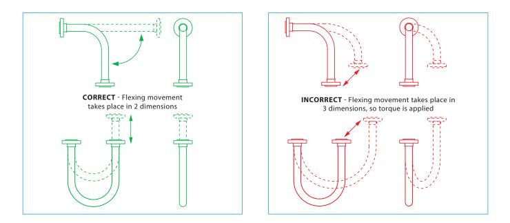
Both Pharmaline and Pharmalex hose have good resistance to a small level of torque, much better resistance that rubber or SS hose types, but it is still the best practice to take whatever steps are necessary to eliminate torque. If in doubt, consult Aflex Hose.
