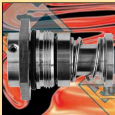
Vulcan manufacture and stock 12mm and 16mm Type 953 screw-fit semi-cartridge seals and 22mm Type 954 push-fit semi-cartridge seals to replace Grundfos® "H-" code seals installed in CR, CRI, CRIE series vertical multi-stage pumps. Type 953 and 954 are intended for all standard clockwise rotation pumps. 16mm Type 953 is also available in "953L" format specifically for "CRI5SF" models with anti-dockwise rotation shafts.
