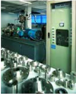
The Vulcan mechanical seal design types shown in this brochure have been tested on our rotary test facilities. The seal performance data produced support Vulcan's published Maximum Recommend Operating Parameters, which can be calculated for each seal type using the provided PV Charts in combination with the Application Conditions and Material Combination Multiplying Factors, please refer to page 16 for a full explanation on how these are calculated.
