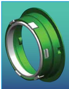
The drive area has been increased by over 250%, to greatly reduce the contact drive pressure and consequent wear. As a result, the drive ring does not cut nor groove into the seal head retainer. The unique seal head design also retains the drive ring by a locking mechanism. This results in security and ease of assembly, due to the unitised design of the entire seal head assembly.
