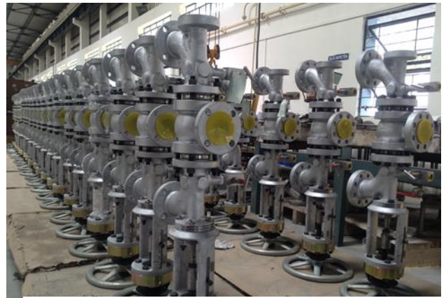
Changeover valves in the workshop
