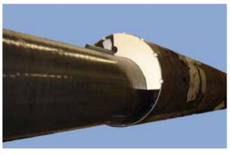
Place foam segments on the carrier pipe and insert into casing pipe. Hereby the raised flange rests on the outer front of the casing pipe. This means that secure support is guaranteed.
