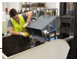
Removable container for disposal of the vacuumed chips
