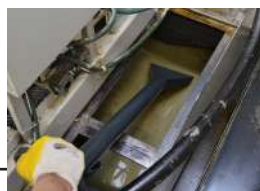
Sludge removal from CNC collection tanks
